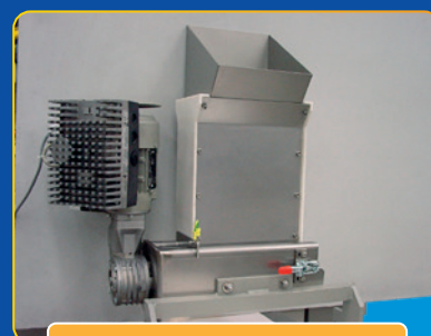
Flour duster for production of sticky- and rye doughs
