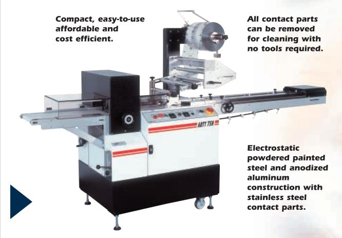
One base model with single, double or quadruple jaws and many attachments to cover a wide variety of wrapping applications.
