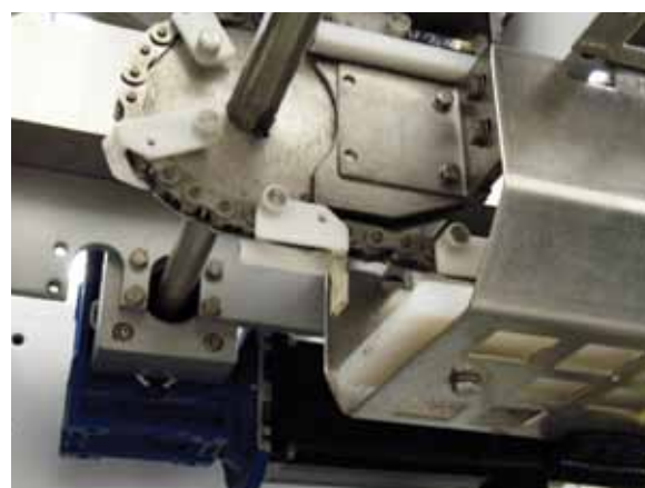
Servo Technology Direct drive design means fewer parts, lower inertia. Linium wrappers run smooth and consistent even under high-speed conditions
